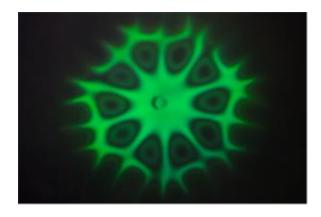
LOE has produced reflective DOEs for CO2 lasers for a number of applications from beam splitting to complex heat profiles for welding applications. Available with a custom mounting box; these optics are very durable and have been industrially proven over many years.
